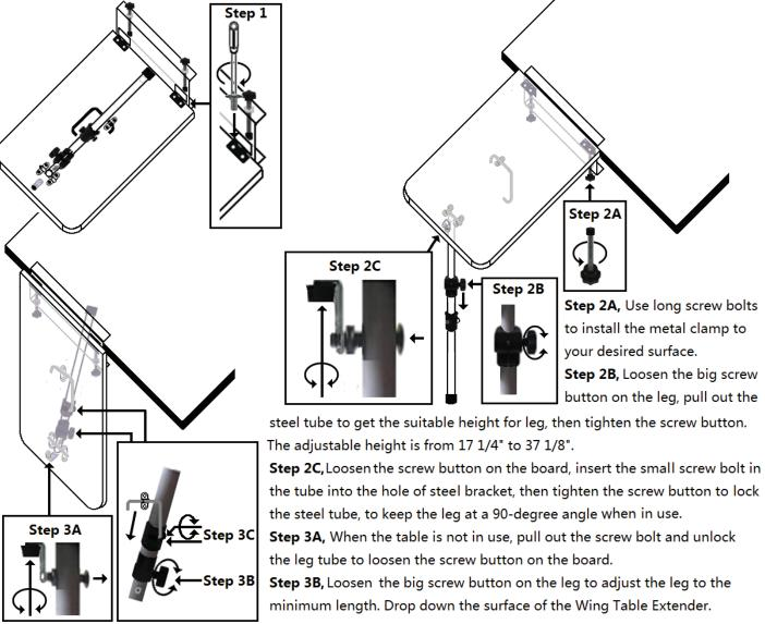
**Step 3C**, Loosen the small screw button on the leg, move the plastic fixing hoop to the suitable position, then insert the steel wire into the hole on the plastic hoop. Tighten the small screw button to fix it.
